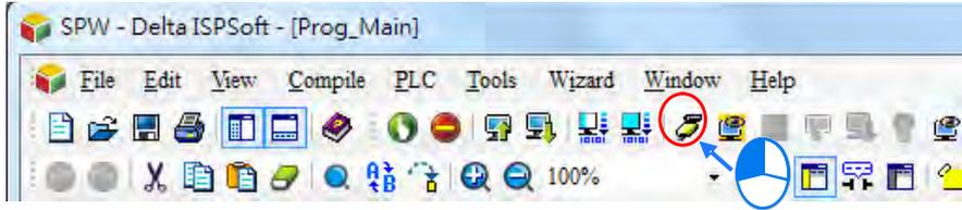
Not only the logic program, but also the information related to the devices is monitored. (If the data type is a Boolean value, the state of the device is represented by green (ON) or white (OFF). If the data type is not a Boolean value, the value in the device is shown.)
