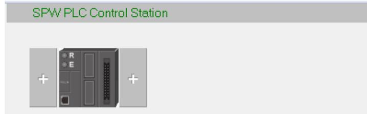
Double-click the CPU module to open the **Device Setting** window.
